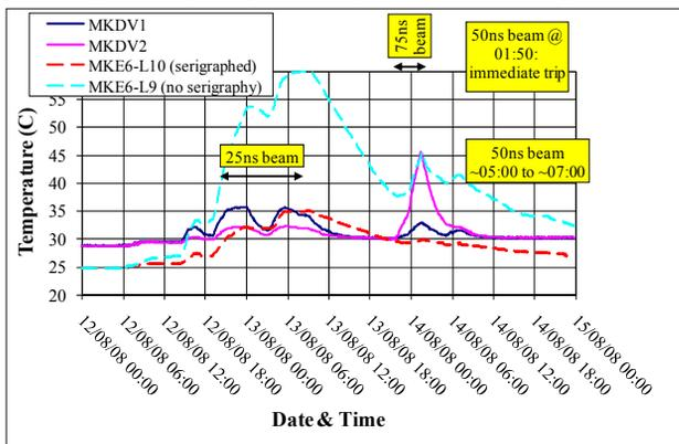
Figure 2: Temperature of MKDV1, MKDV2 and two MKE6 magnets during MD of 12 to 14 August, 2008.
