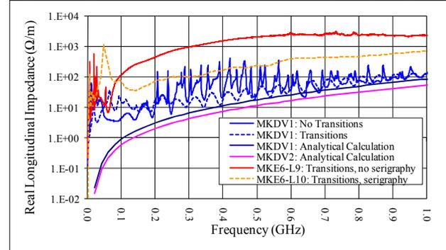
Figure 3: Analytical RLCI for MKDV1 & MKDV2 & measured RLCI for MKDV1 & 2 MKE6 kicker magnets.
