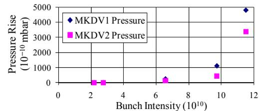
Figure 7: Pressure rise in MKDV kickers versus bunch intensity (50 ns bunch spacing and 4 batches).
