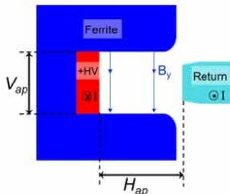
Figure 1: Simplified cross-section of a kicker magnet.
