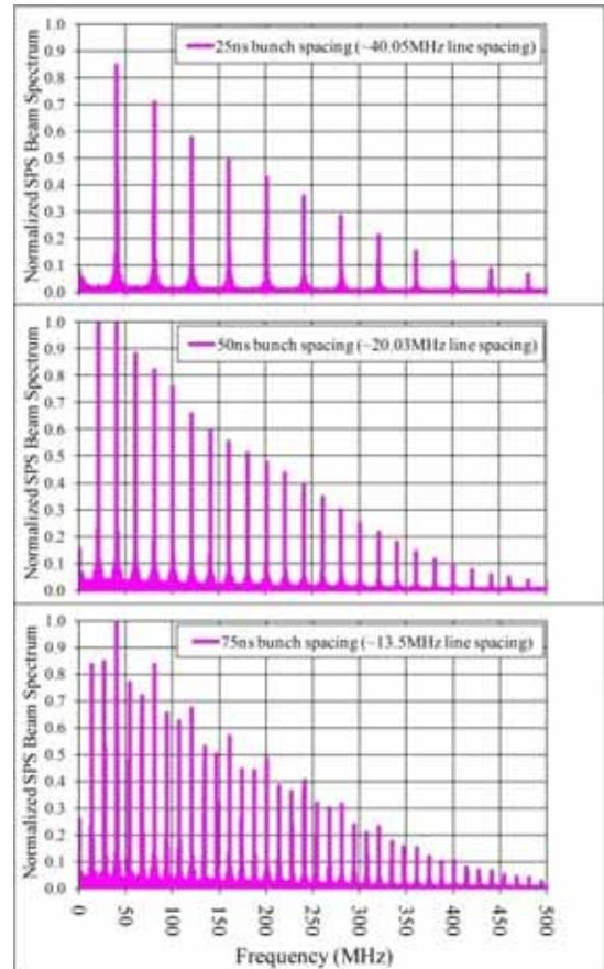
Figure 4: Normalized, measured, SPS beam spectrum for 25 ns, 50 ns and 75 ns bunch spacing.
