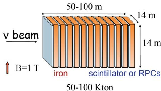
Figure 2: (Color) Schematic of the MIND concept for the Neutrino Factory.
