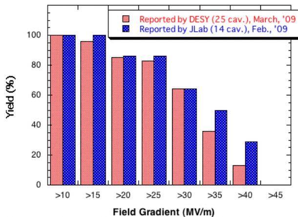
Figure 1: Recent status of global cavity yield (DESY 25 cavities [6], and JLab 14 cavities [7]). Datasets represent cavities from more than one vendor. Majority of results represent first vertical test (second test in a few cases).
