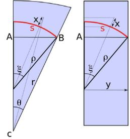
Figure 1: difference of geometry in circular ring element (left) and in straight section element (right).
