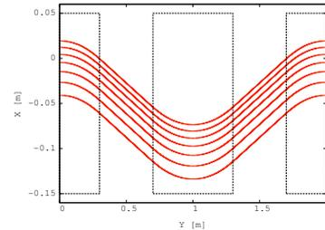
Figure 2: reference trajectories for kinetic energies from 80 MeV (bottom) to 200 MeV (up).
