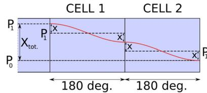
Figure 4: Dispersion suppressor made of 2 cells with 180-degree phase advance each. Dotted lines show intrinsic reference trajectories of the cells, and red line shows the distortion of reference trajectories generated by the difference  $x$ .
