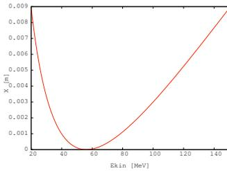
Figure 3: difference of reference trajectories between circular cells and straight cells in 150 MeV FFAG ring example.
