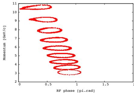
Figure 3: 8 turns acceleration cycle plotted in the longitudinal phase space, at the location of cavity number 0. Initial beam emittance is  $0.21 \text{ eV.s} \times 10\,000 \pi \text{ mm.mrad}$  (normalized).
