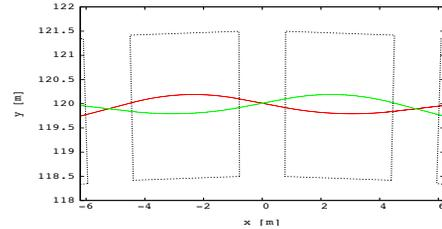
Figure 2: Closed orbits of  $\mu^+$  and  $\mu^-$  circulating in the same direction. Results are obtained from Runge-Kutta stepwise tracking in hard-edge field.
