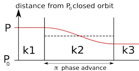
Figure 5: Principle of excursion reducer  $\pi$  section.
