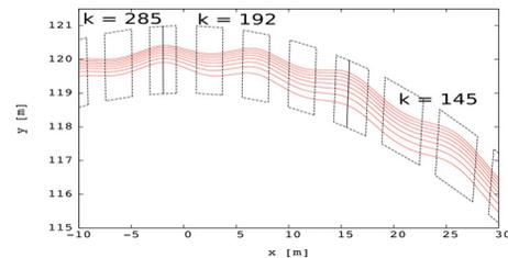
Figure 6: Here excursion is reduced from 0.98m to 0.50 m with the help of a  $\pi$  section with  $k = 192$ .
