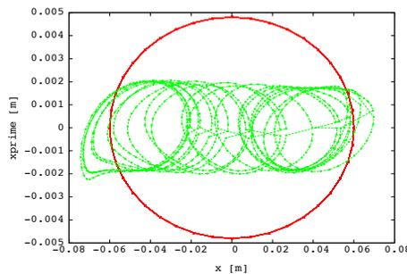
Figure 4: First turn (red squares) and last turn (green dots) of the 8 turns acceleration cycle plotted in transverse phase space. Beam emittance is  $0.21 \text{ eV.s} \times 10\,000 \pi \text{ mm.mrad}$  (normalized). The horizontal beam spread of the last turn is due to the effect of dispersion (beam is not mono-energetic).
