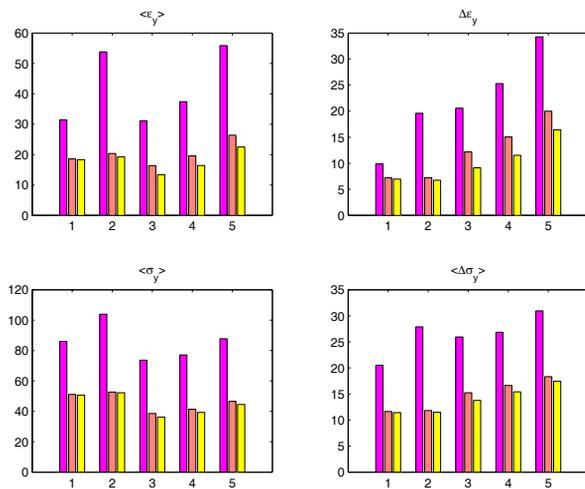
Figure 1: Vertical emittance (upper figures) and vertical beam size (lower figures) comparison with different sets of input errors.
