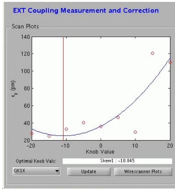
Figure 2: Vertical emittance reconstructed from multi-wire beam size measurements as a function of QK1X strength.
