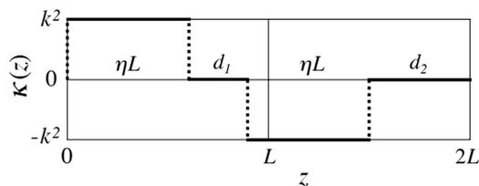
Figure 1: Model for  $xz$ -plane in one cell of a periodic FoDO lattice. The quadrupoles have equal lengths  $\eta L$ ; gap lengths are  $d_1$  and  $d_2$ . The cell starts at  $z = 0$  with  $\kappa > 0$  (focus). The  $yz$ -plane field map is the same but inverted.
