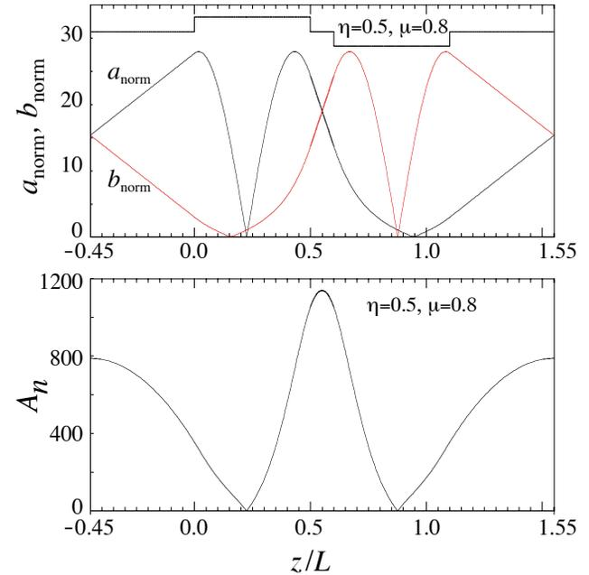
Figure 6: Normalized  $a(z), b(z)$ , and  $A_n(z) \equiv \pi ab$  near outer edge of band 2:  $kL = 2.41361\pi$ ;  $\sigma = 356.6^\circ$ . The beam compression ( $7 \times 10^4$ ) is reduced because the gaps have unequal length and the  $a(z)$  and  $b(z)$  minima do not coincide—see text.
