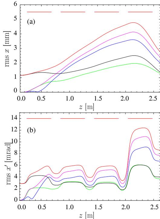
Figure 4: (Color) rms centroid coordinate  $x$  (a) and angle  $x'$  (b) for an ensemble of errors and  $B_{\max} = 2.6, 1.4, 1.06,$  and  $2.35$  Tesla. Key: Red (All), Magenta ( $\Delta_{x,y}$  and  $\Theta_{x,y}$ ), Blue ( $\Theta_{x,y}$ ), Green ( $\Delta_{x,y}$ ), Black (initial  $x, x', y, y'$ )
