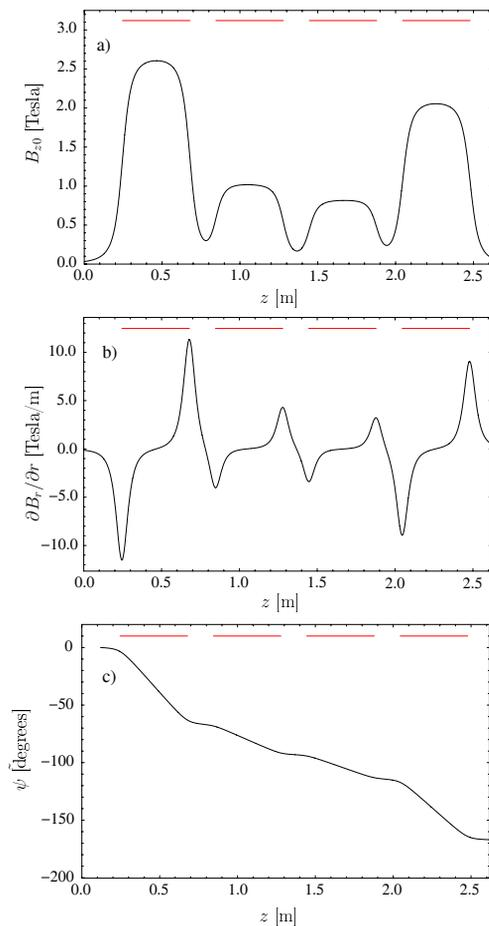
Figure 3: (Color) Axial magnetic field  $B_{z0}$  (a), transverse magnetic field gradient  $\partial B_r/\partial r$  (b), and Larmor frame rotation angle  $\tilde{\psi}$  (c) versus axial coordinate  $s$ .
