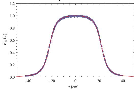
Figure 2: (Color) Best fit of the thin coil model (red curve) to measured solenoid data (blue dots).
