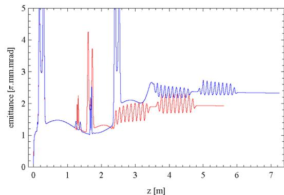
Figure 3: Normalised transverse emittance (rms) along the existing (red) and extended (blue) injector beamlines.
