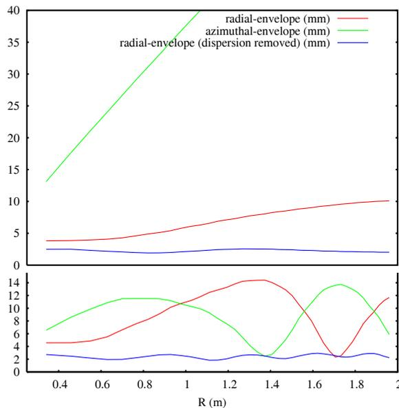
Figure 2: Beam being accelerated in a cyclotron, envelopes as function of  $R$ ; initial bunch length = 10 mm (upper), and 5 mm (lower). The parameters correspond to the TRIUMF 500 MeV cyclotron:  $R_\infty = 10$  m, so the energy range on this plot is from 0.3 to 20 MeV; 50 turns since  $\Delta E = 0.4$  MeV/turn.
