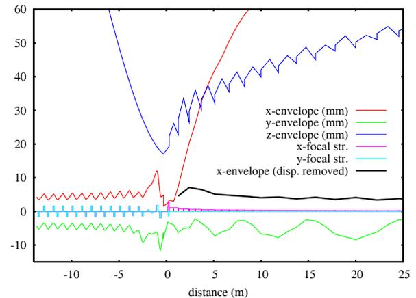
Figure 3: Beam envelopes through the injection line and into the cyclotron. Charge per bunch is  $22 \text{ pC}$  for a time average current  $0.50 \text{ mA}$ .
