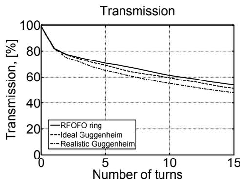
Figure 3: Transmission (number of particles in the beam after a number of turns).
