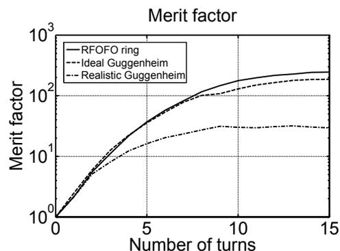
Figure 5: Merit factor (inverse ratio of six-dimensional emittances multiplied by transmission).
