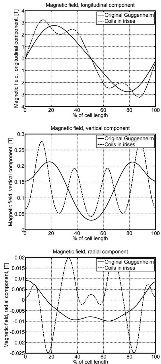
Figure 8: Magnetic field comparison between the RFOFO ring (or Guggenheim, fields are very similar) and the new layout, one cell shown.
