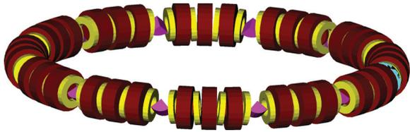
Figure 6: New cooling channel layout with magnetic coils in the irises of the RF cavities
