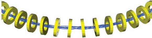
Figure 7: Solenoid axes are tipped  $4.9^\circ$  above or below the orbital midplane depending on the direction of the current.
