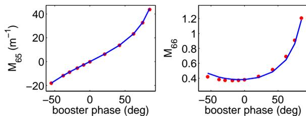
Figure 4:  $M_{65}$  (left) and  $M_{66}$  (right) element of the transfer matrix of the booster cavity in the longitudinal phase space  $(z, \delta)$ . The simulated transfer matrix using IMPACT-T (red symbols) is compared with analytical calculation (blue lines).
