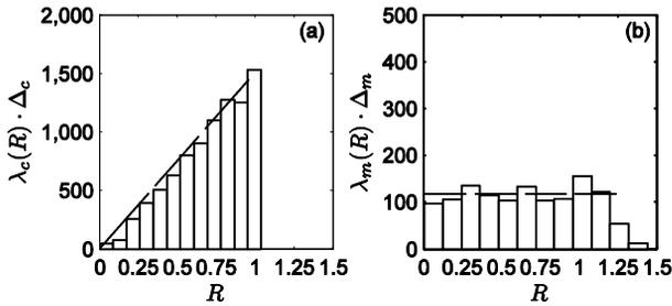
Figure 3: Histograms for beam particle density computed through numerical simulations (bins) and the exact analytical model (solid line). Comparison occur in panel (a) for beam core with  $\Delta_c \cong 0.0866$  and in panel (b) for beam halo  $\Delta_m \cong 0.1194$ . Magnitude of inhomogeneity  $\eta = 0.5$ .
