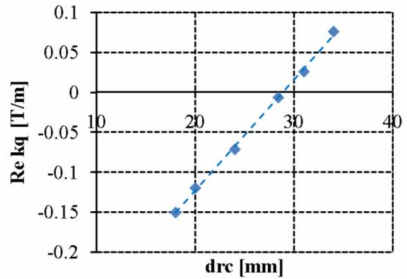
Figure 5: Real part of the dipole component with the distance of the racetrack centers.
