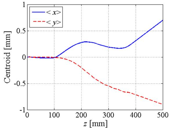
Figure 8: Centroid of the beam. The blue, solid line is that of horizontal (the input port direction) distribution and the red, dashed line is that of the vertical one.
