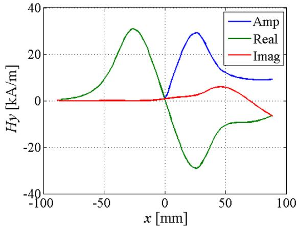
Figure 7:  $H_y$  along the coupler center from the dummy port to the input port. The blue line shows the amplitude of  $H_y$ , green the real part, and red the imaginary part.
