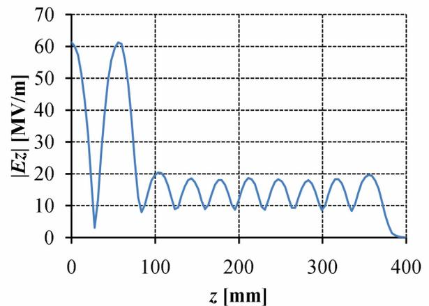
Figure2: Amplitude of the electric field on the beam axis.
