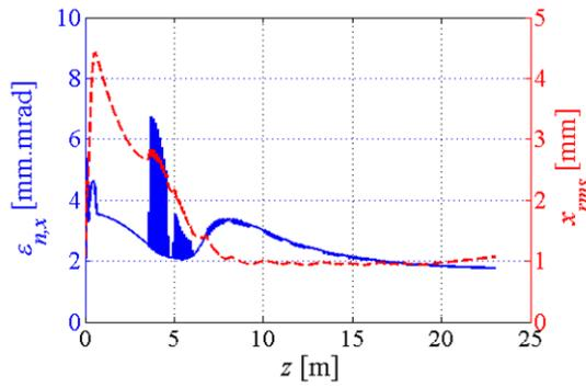
Figure 3: The horizontal normalized emittance (blue, solid line) and beam envelope (red, dashed line) along  $z$  for 1 nC bunch with mild compression.
