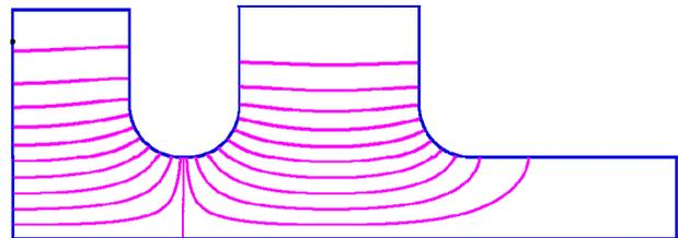
Figure 2: The shape of the 1.6-cell RF gun.
