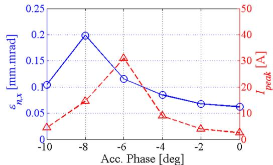
Figure 8: The horizontal normalized emittance (blue, solid line and circle markers) and the peak current (red, dashed line and triangle markers) with the phase in the first linac for 1 pC bunch.
