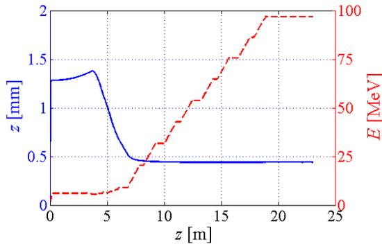
Figure 5: The rms of bunch length (blue, solid line) and the energy (red, dashed line) along  $z$  for 1 nC bunch with mild compression.
