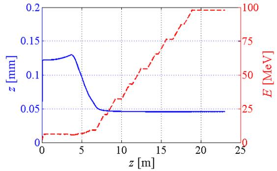
Figure 6: The rms of bunch length (blue, solid line) and the energy (red, dashed line) along  $z$  for 1 PC bunch with mild compression.
