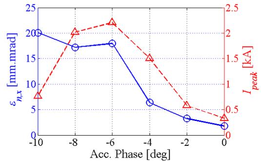
Figure 7: The horizontal normalized emittance (blue, solid line and circle markers) and the peak current (red, dashed line and triangle markers) with the phase in the first linac for 1 nC bunch.
