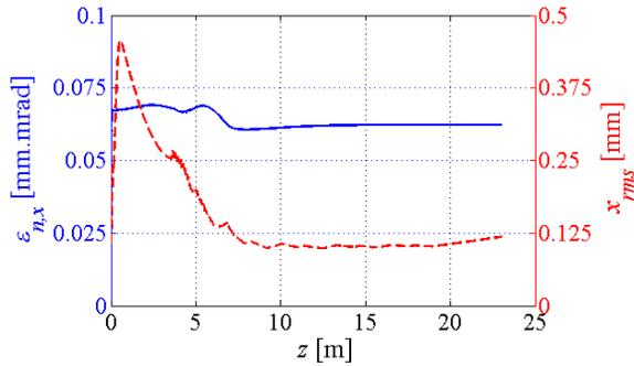
Figure 4: The horizontal normalized emittance (blue, solid line) and beam envelope (red, dashed line) along  $z$  for 1 pC bunch.
