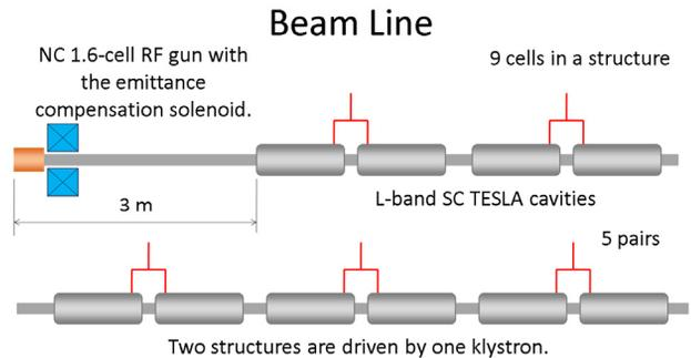
Figure 1: The layout of the beamline for the simulation.
