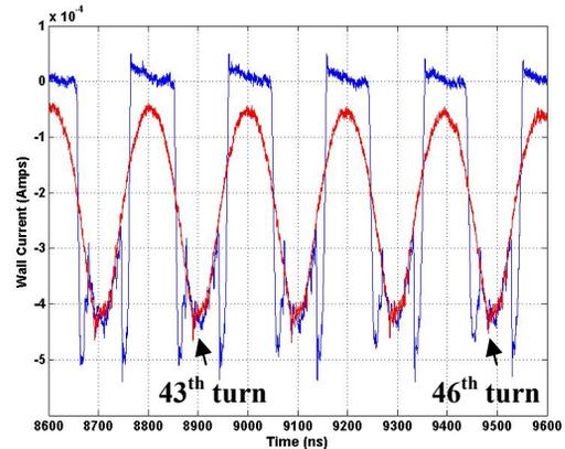
Figure 8: Long term effects of longitudinal focusing (Red-no focusing, Blue- with focusing).
