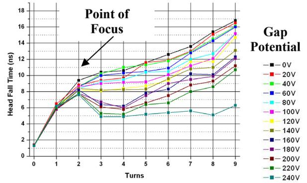
Figure 4: Beam head fall times with single application of focusing on 2<sup>nd</sup> turn as a function of turns and Gap potential, measured at RC10.
