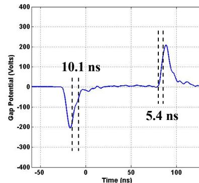
Figure 2: Gap potential as a function of time for both the decelerating and accelerating focusing field.
