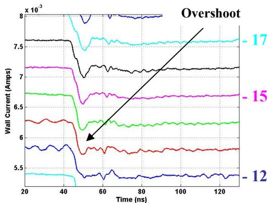
Figure 7: Overshoots in beam current measured at RC10.
