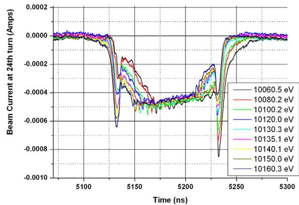
Figure 5: Beam current measured on the 24<sup>th</sup> turn at RC10, as function of swept energy.
