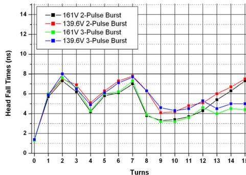
Figure 6: Beam head fall times measured at RC10.
