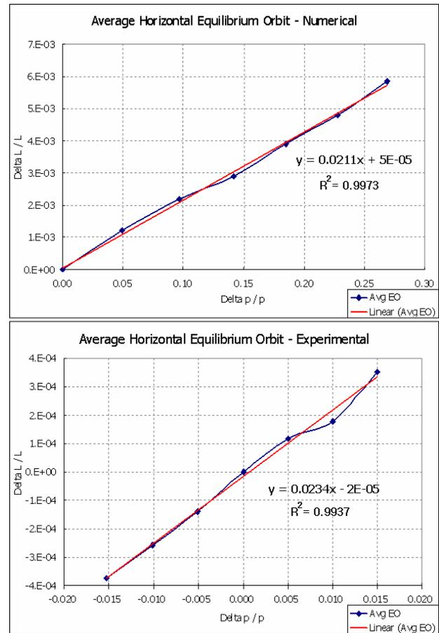
Figure 4: Comparison among numerical and experimental results for momentum compaction, by fitting data of the average of the horizontal equilibrium orbit as function of variation on momentum.
