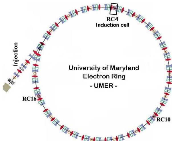
Figure 1: University of Maryland Electron Ring layout, showing the actual induction cell location at RC4, and the places for two additional induction cells at RC10 and RC16. The total circumference of the ring is 11.52 m, and the induction cells are equally distant from each other.
