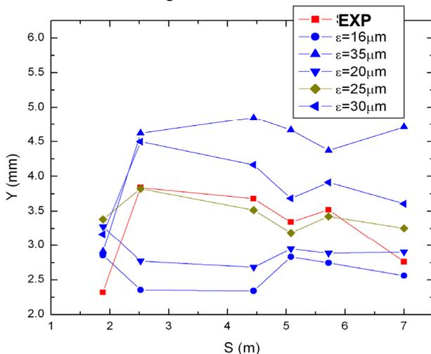
Figure 3: 2\*rms Y envelope of the 7 mA beam in the ring: experiment (red) vs. WARP simulations assuming different initial emittance values. Settings of matching method B.
