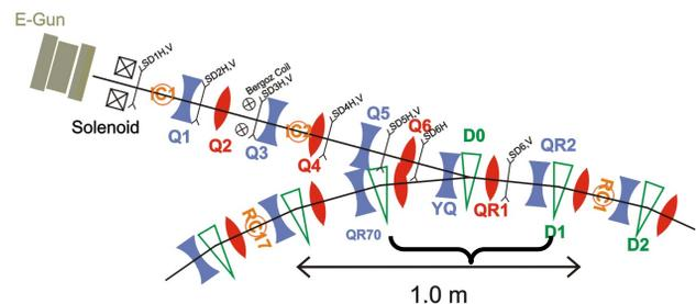
Figure 1: Schematic of the UMER injection line.
