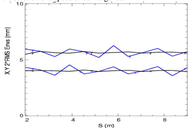
Figure 2: x-y beam envelopes in the diagnostic chamber locations before (blue) and after (black) simulated empirical matching of the 23 mA beam.
