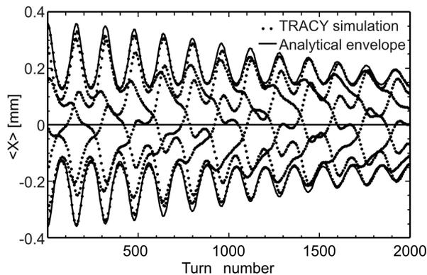
Figure 2: TRACY simulation (dots) and envelope calculated by the analytical formula (14) (solid line).
