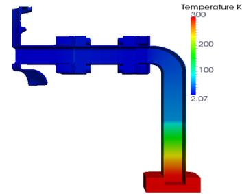
Figure 3: Temperature field caused by EM heating.
