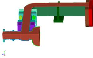
Figure 1: The CAD model of JLAB SCRF cavity including metal and vacuum region.
