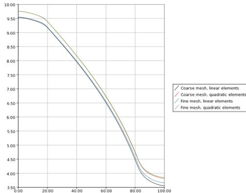
Figure 5: Temperature along a line using different meshes, and FEM discretization.
