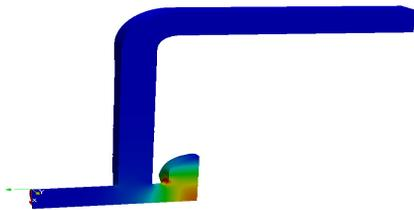
Figure 2: Electric field distribution for the accelerating mode..
