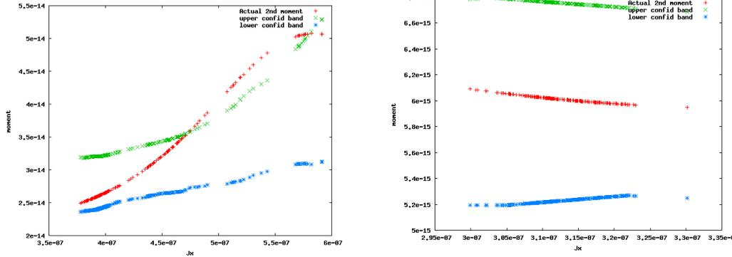
Figure 1: (left) The evolution of the second moment as the action nears the dynamic aperture at  $6\sigma$  initial transverse horizontal (X) action in a RHIC simulation with both long-range and head-on kicks. The diffusion ceases to be regular beyond the dynamic aperture. (right) The evolution of the second moment below the dynamic aperture at  $5\sigma$  initial transverse horizontal (X) action in a RHIC simulation with both long-range and head-on kicks. The diffusion appears regular.
