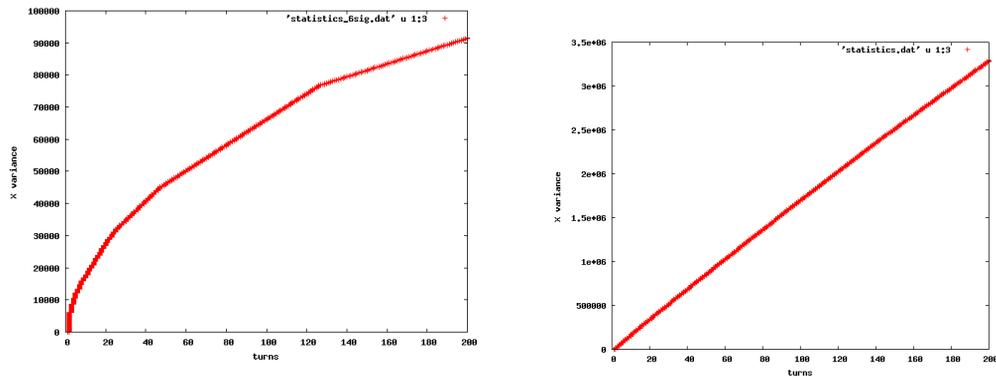
Figure 2: (left) The time dependence of the variance at  $6\sigma$  initial action. The diffusion ceases to be regular since the time dependence is not linear  $H \neq 1/2$  (agrees with results of simulated paths). (right) The time dependence of the variance at  $5\sigma$  initial action. The diffusion should be regular since the time dependence is clearly linear  $H = 1/2$  (agrees with results of simulated paths).
