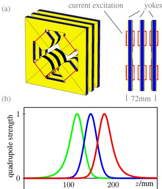
Figure 2: (a) Different views on a schematic computational model of a compact quadrupole triplet as used at the S-DALINAC. In (b) the extracted normalized quadrupole strength of each individual magnet is displayed.
