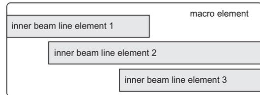
Figure 3: Scheme of an enveloping macro element with three overlapping inner beam line elements.
