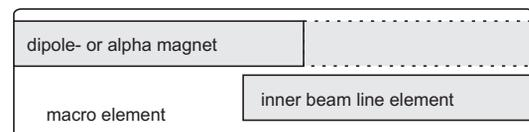
Figure 4: Scheme of a dipole- or alpha magnet enveloping macro element together with an overlapping inner beam line element.
