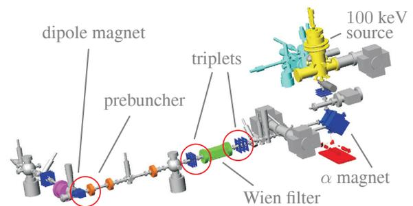
Figure 1: Schematic computational model of the compact injector design for the new polarized electron source at the S-DALINAC. Selected areas with overlapping fringe fields are marked by circles.
