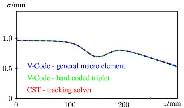
Figure 7: Simulation of the vertical focusing effect within the compact quadrupole triplet shown in Fig. 2
