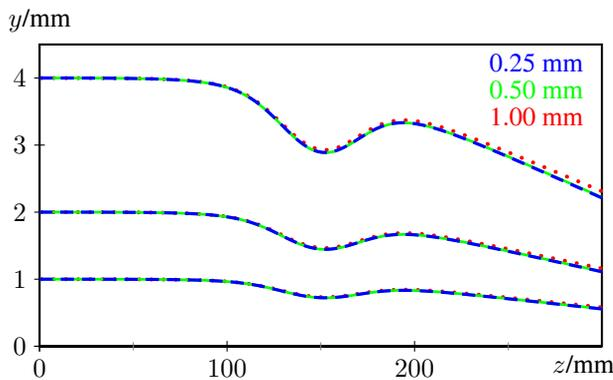
Figure 5: Trajectories of single particles with vertical offset of 1, 2 and 4 mm within the compact quadrupole triplet shown in Fig. 2. The results of simulations with the CST particle tracker on different mesh densities (0.25, 0.5 and 1mm) are displayed.
