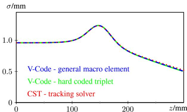
Figure 6: Simulation of the horizontal focusing effect within the compact quadrupole triplet shown in Fig. 2
