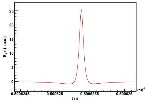
Figure 2: The calculated electric pulse due to an electron in a circular orbit. The observation point is in the same plane as the electron's path, so only the  $x$ -component of the electric field is present.
