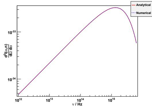
Figure 3: The differential power spectrum for an electron in a circular orbit, measured in  $\text{J Sr}^{-1}$ , radiated into unit frequency interval. The analytical and numerical curves agree within 0.05%.
