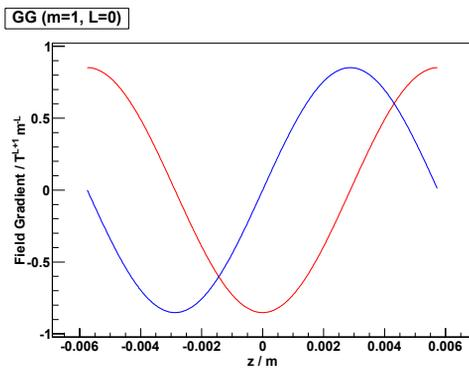
Figure 5: The normal (red) and skew (blue) dipole components of the generalised gradients  $C_{1,s}^{[0]}$  and  $C_{1,c}^{[0]}$  for the helical undulator. These components are identified with the on-axis fields  $B_y$  and  $B_x$ .
