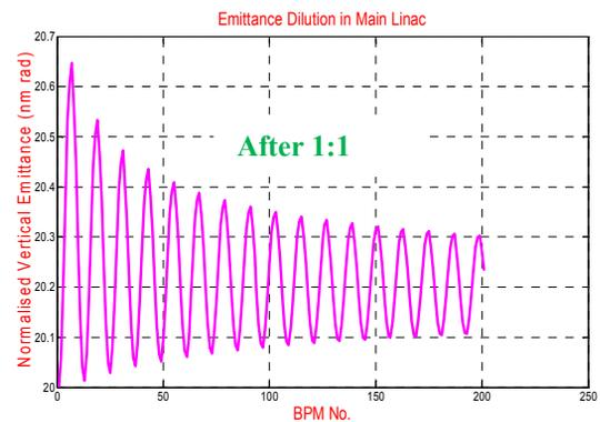
Figure 4: Emittance behaviour of the beam after 1:1 correction in Main Linac when only imaginary part of voltage ( $V: 0.0+i 11.1$ ) is applied to TCAV.
