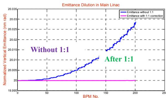
Figure 2: Emittance behaviour of the beam in the Main Linac when only real part of kick voltage is applied to TCAV ( $V: -7.3 + i0.0$ ). Effect of 1:1 correction is also shown.
