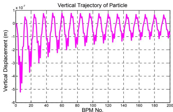
Figure 7: Trajectory of Particle under the influence of Coupler wake field.
