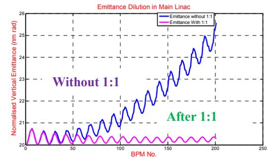
Figure 5: Emittance behaviour of the beam in Main Linac when both real & imaginary part of kick voltage ( $V: -7.3+ i 11.1$ ) is applied to TCAV.
