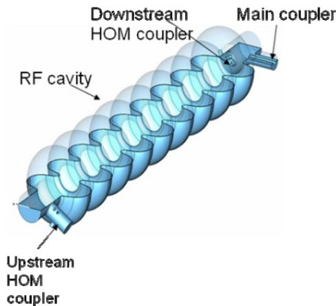
Figure 1: The ILC RF cavity with main & HOM couplers.
