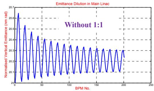
Figure 3: Emittance behaviour of the beam along the Main Linac when only imaginary part of kick voltage ( $V: 0.0+i 11.1$ ) is applied to TCAV.
