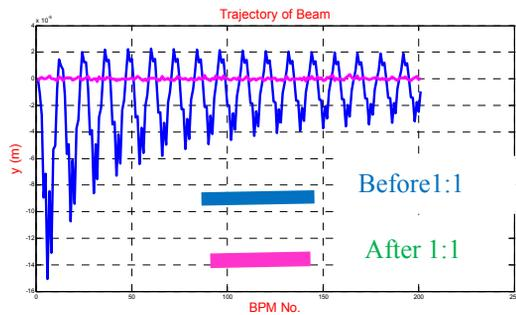
Figure 6: Vertical Trajectory of the beam in the main linac when both real & imaginary part of kick voltage (V:-7.3+ i 11.1) is applied to TCAV. Effect of 1:1 correction is also shown.
