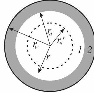
Figure 1: Cross-section of a cylindrical DLA structure. 1 – vacuum region, 2 – dielectric,  $r_d$  – radius of dielectric,  $r_w$  – radius of waveguide wall,  $r'_n$  – location of the charged layer.
