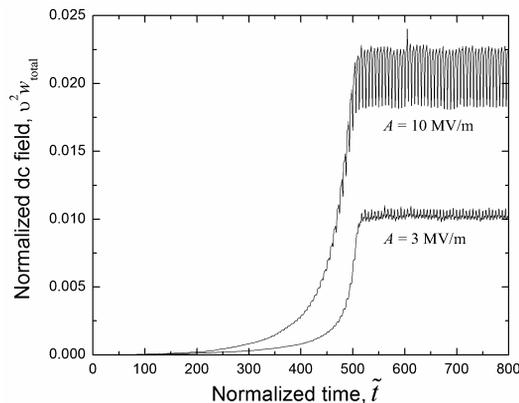
Figure 2: Number of macroparticles (a) and normalized total dc field (b) as functions of time for two values of the rf amplitude.
