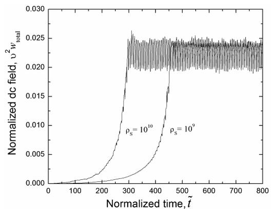
Figure 4: Normalized total dc field as function of time for two values of the seed particle density. The rf amplitude is equal to 10 MV/m in both cases.
