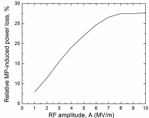
Figure 3: Ratio of MP-induced loss to power flowing in the structure as function of the rf amplitude. Calculations are done for a 20 cm long structure shown in Fig. 1 of Ref. 1.
