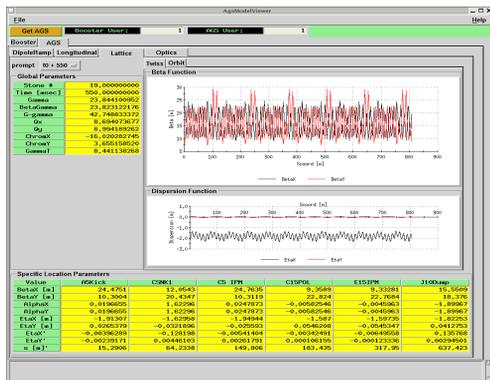
Figure 1: AgsModelViewer showing lattice functions calculated by online model.
