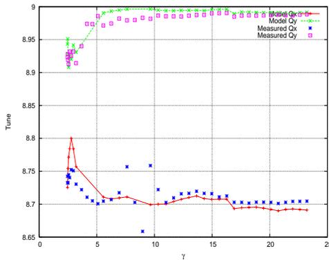
Figure 3: Betatron tune model predictions and measurement for polarized proton operation in the AGS.
