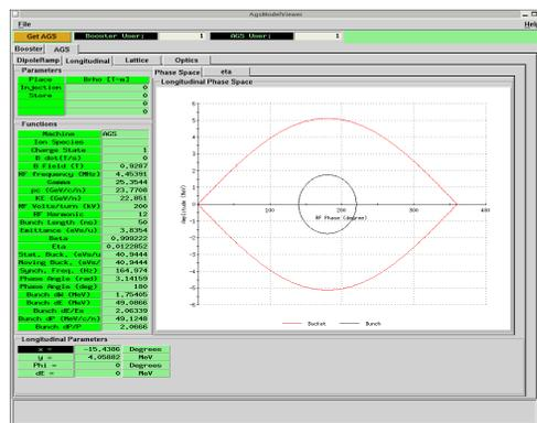
Figure 2: AgsModelViewer showing longitudinal phase space calculated by online model.
