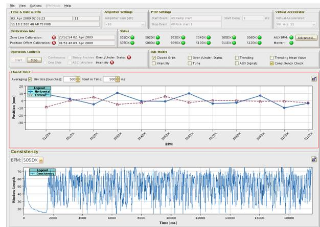
Figure 4: Java GUI showing first orbit data recorded with the new SIS-18 BPM system.
