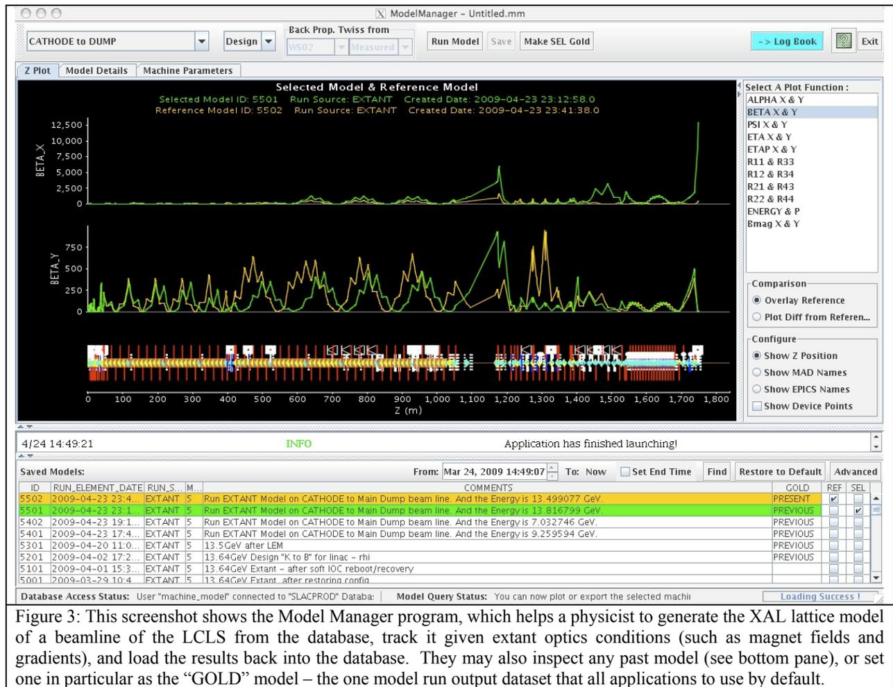
Figure 3: This screenshot shows the Model Manager program, which helps a physicist to generate the XAL lattice model of a beamline of the LCLS from the database, track it given extant optics conditions (such as magnet fields and gradients), and load the results back into the database. They may also inspect any past model (see bottom pane), or set one in particular as the “GOLD” model – the one model run output dataset that all applications to use by default.
