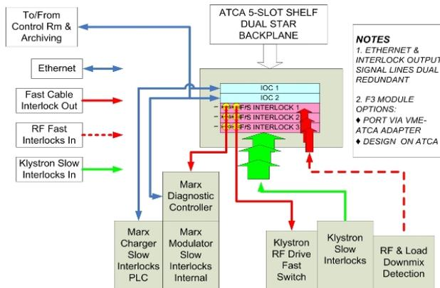
Figure 2: Simplified Block Diagram – Phase II.
