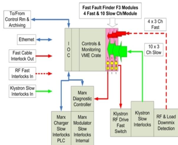
Figure 1: RF Controls and Interlocks Simplified Block Diagram – Phase I.
