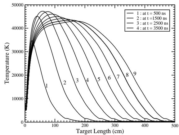
Figure 3: Temperature along the axis (at  $r=0.0$ ) at different times during irradiation, time interval between two consecutive lines is  $1 \mu s$ .
