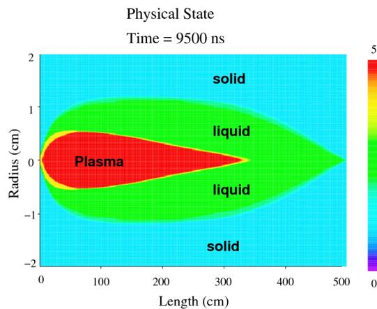
Figure 6: Physical state of the target shown at  $t = 9.5 \mu\text{s}$ .
