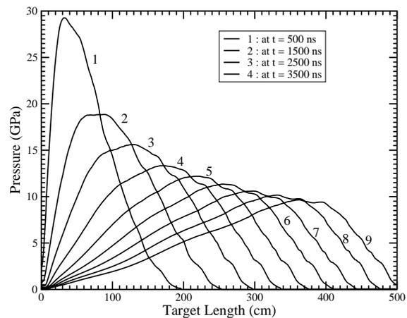
Figure 4: Pressure along the axis (at  $r=0.0$ ) at different times during irradiation, time interval between two consecutive lines is  $1 \mu s$ .
