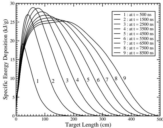
Figure 2: Specific energy deposition along the axis (at  $r = 0.0$ ) at different times during irradiation, time interval between two consecutive lines is  $1 \mu s$ .
