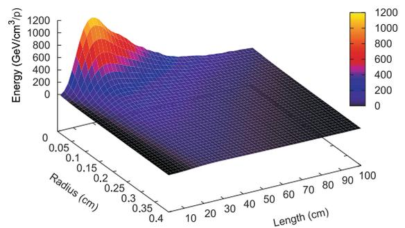
Figure 1: Energy deposition in a solid copper cylinder by a single 7 TeV proton per unit volume.
