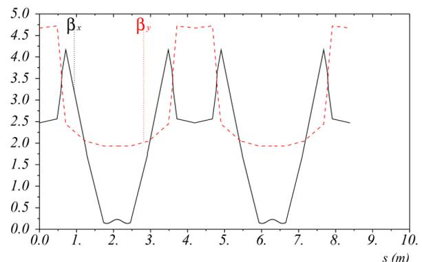
Figure 2: Lattice function as calculated with MAD.
