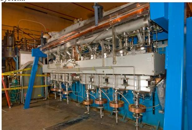
Figure 4: Cavity string suspended from the lid, with all cryogenic plumbing assembled and leak-checked, ready to drop into the box vacuum vessel.
