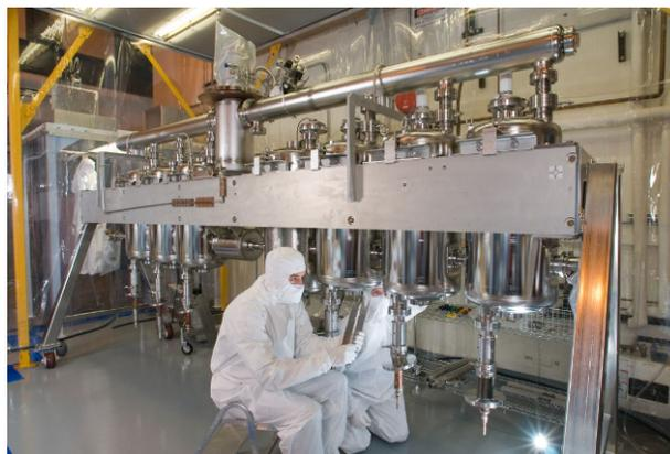
Figure 3: The cavity string assembly in the clean area is complete, including complete, sealed cavity vacuum system.
