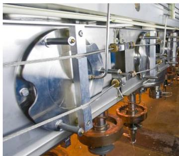
Figure 2: Slow tuners mounted on the cavities.
