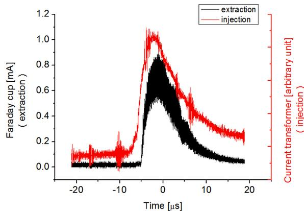
Figure 7: Beam pulse profiles.
