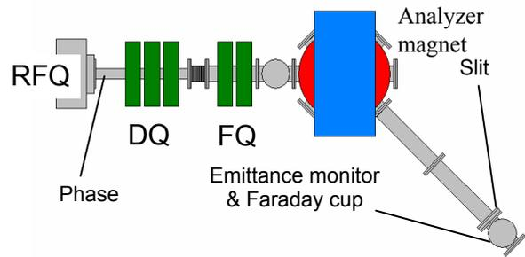
Figure 8: A beam line for analyzing multi charged ions.
