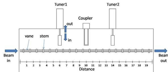
Figure 1: Frequency tuners and RFQ vanes.
