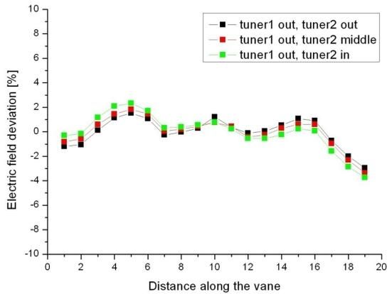
Figure 3: Field distribution along the beam axis.
