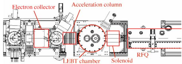
Figure 5: Injection beam line to the RFQ.
