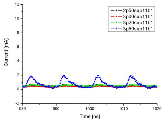
Figure 6a: Measured current after the RFQ at lower RF power.
