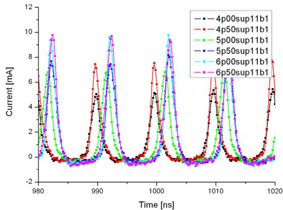
Figure 6b: Measured current after the RFQ at higher RF power.
