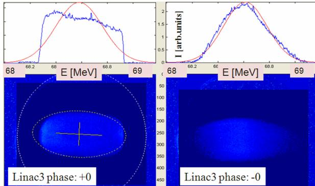
Figure 3: Zero-phasing with Linac3. Lower plots are beam images on the BPM. Upper are energy projections (blue), and Gaussian fits (red).
