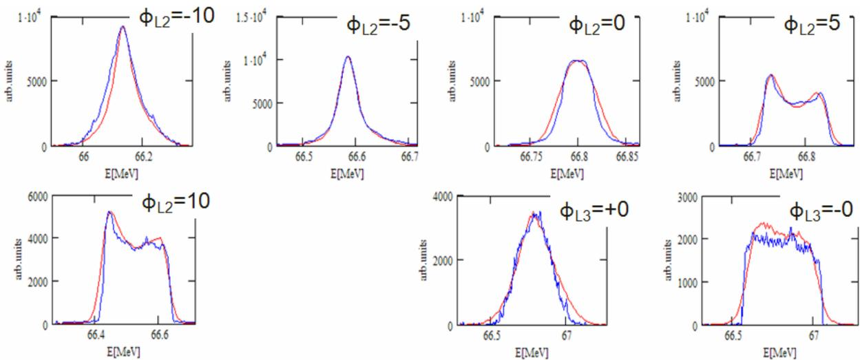
Figure 4: Simplified tomography. Blue traces represent measured 50pC beam projections on energy axis for Linac2 scan (first 5 plots) and for Linac3 zero-phasing (2 last plots); measured projections are fit (red) with simulated beam distribution shown in Fig. 5.
