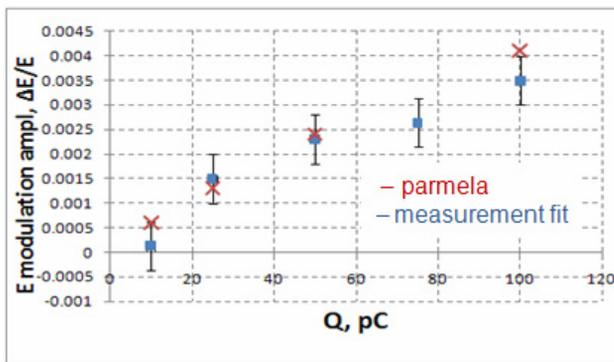
Figure 6: Measured (blue) and PARMELA simulated (red) energy modulation of 100fs, 10pC-100pC beam.
