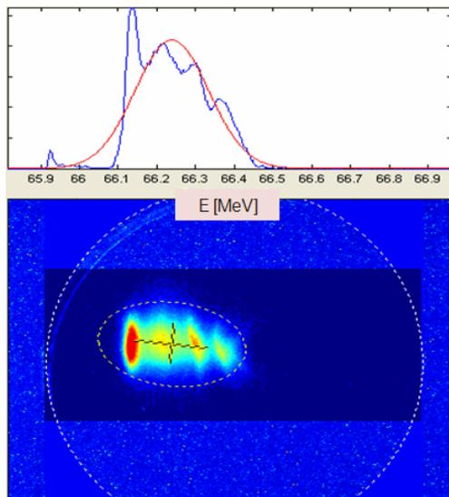
Figure 7: Beam substructures at nominal chicane settings and -20deg off-crest Linac2 phase. Lower plot is beam image on the BPM. Upper is energy projection.
