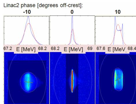
Figure 2: The scan of Linac2 phase. Lower plots are beam images on the BPM. Upper are energy projections (blue), and Gaussian fits (red).
