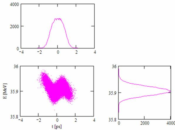
Figure 5: Beam's longitudinal phase space at the entrance of Linac2 reconstructed with simplified tomography. Chirping this distribution produces pseudo-structures in energy domain.
