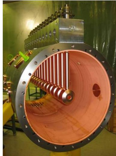
Figure 4: DTL prototype.
