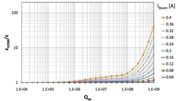
Figure 1: Effective emittance growth rate versus  $Q_{ex}$  for different beam currents assuming one HOM per cavity ( $\sigma_f = 0.1$  MHz,  $\sigma_I = 10\%$ ).
