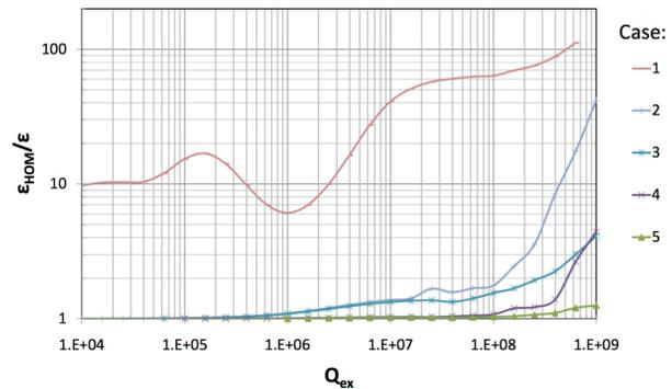
Figure 3: Effective emittance growth rate of the beam against  $Q_{ex}$  for the 5 different scenarios listed in Table 4.
