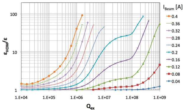
Figure 2: Effective emittance growth versus  $Q_{ex}$  for different beam currents with one HOM per cavity next (1 MHz) to a machine line ( $\sigma_f = 0.1$  MHz,  $\sigma_I = 10\%$ ).
