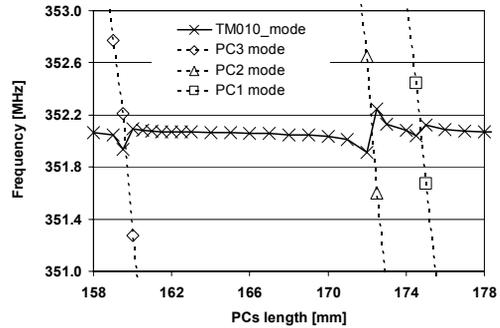
Figure 5: Measurements showing PC modes crossing  $TM_{010}$  mode.
