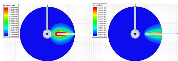
Figure 7: E and H field magnitude of the  $PC_1$  mode.
