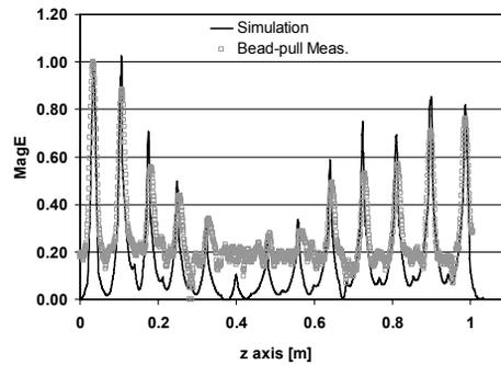
Figure 6: Simulated and measured field on axis for the highest PC mode ( $PC_1$  mode).
