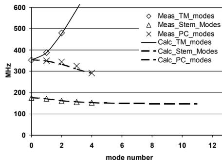
Figure 9: Calculated and measured dispersion curves for TM modes, PC modes and stem modes (PC length = 178 mm).
