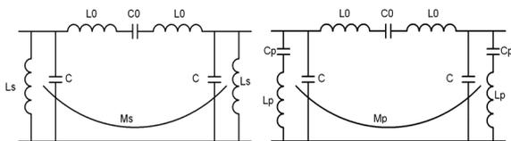
Figure 8: Equivalent circuit of a basic DTL cell with stems (left) or PCs (right).
