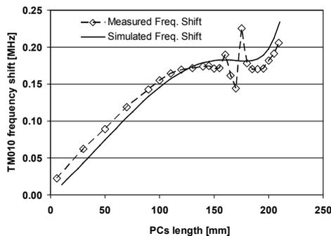
Figure 4: Simulated (Superfish) and measured  $TM_{010}$  detuning as function of PC length.
