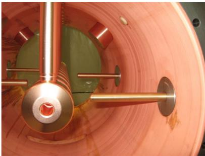
Figure 1: DTL hot prototype, internal view with PCs.
