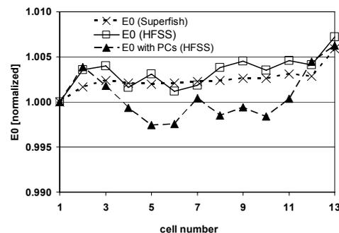
Figure 2: Average E field on axis as computed by Superfish and by HFSS, without and with PCs.
