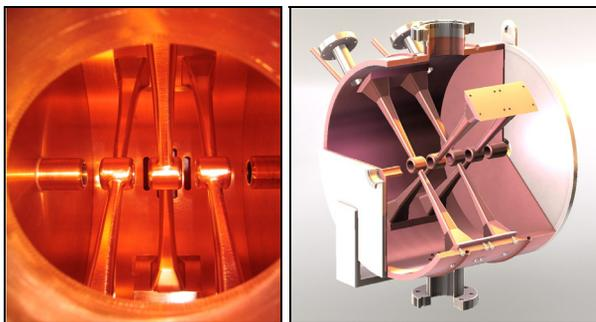
Figure 2: HINS RT-CH cavities: 3-spoke cavity photograph and 4-spoke cavity design rendering.
