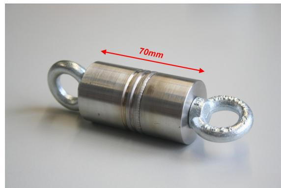
Figure 5: Prototype to test a stress relaxation concept used at the stem ends.
