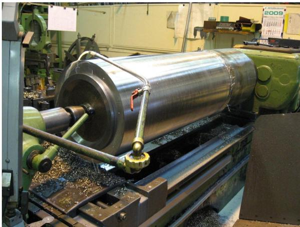
Figure 7: Milling of the outer cylindrical wall at one part of the prototype cavity and preparation for thrilling the longitudinal water cooling channels.
