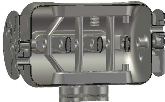
Figure 2: Design of the superconducting 7-cell CH-Cavity (325 MHz,  $\beta = 0.16$ ).
