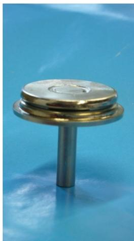
Figure 4: Prototype of the membrane tuner.
