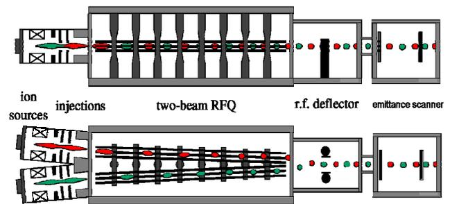
Figure 2: Scheme of the experimental setup.
