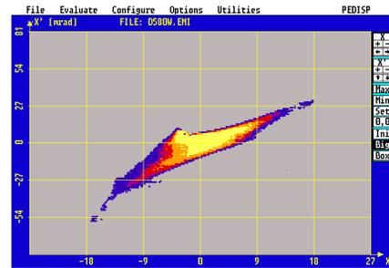
Figure 7: Beam measurement with switched on deflector
