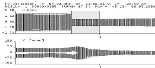
Figure 5: Simulation of the beam bending in the one cell funnel deflector.
