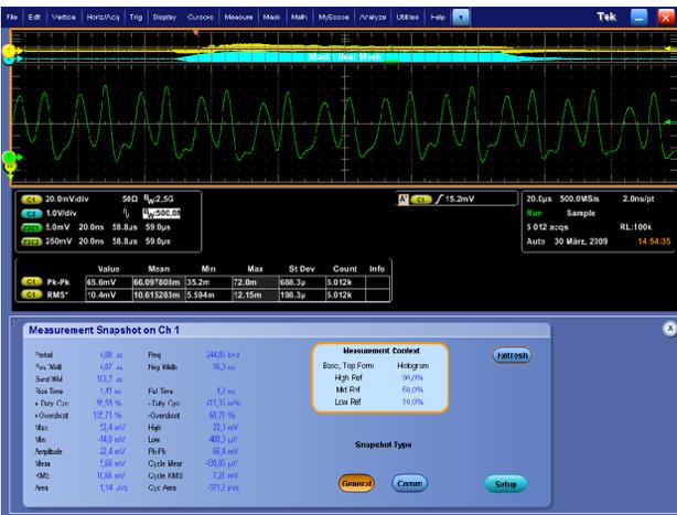
Figure 10: Micropulse measurement with a fast Faraday cup
