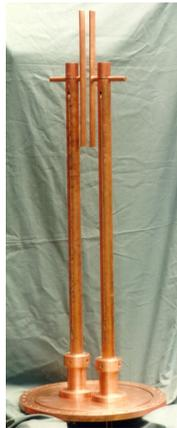
Figure 4: Picture of the one cell funnel deflector. The deflector discs are mounted at water-cooled stems. The height is about 2 m.
