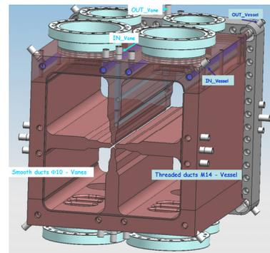
Figure 2: The cooling ducts lay out for an Half Module. There are independent threaded ducts (M14) for the vessel and smooth ducts in parallel (D10) for the vanes.
