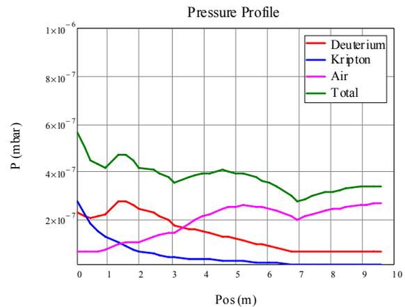
Figure 8: Pressure profile along the RFQ.
