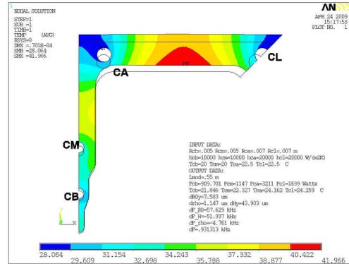
Figure 5: Temperature map in the 2D section in the highest power zone.
