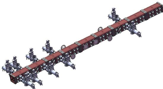
Figure 7: Schematic layout of the vacuum system for the RFQ. The beam comes from the left to the right. Section at beam entrance has 8 pumps, Middle section has 8 couplers, the end section has 2 pumps.
