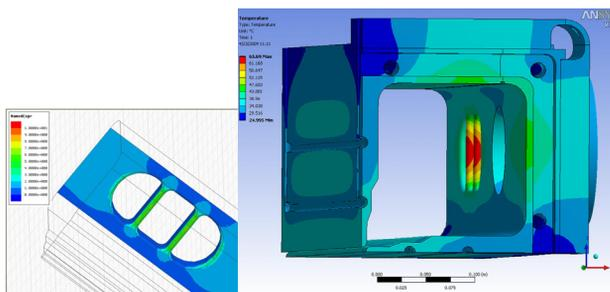
Figure 6: Power density normalized to the 2D max value  $p_0=5.5$  W/cm<sup>2</sup> (LEFT). Temperature map in the vacuum port (RIGHT).
