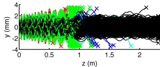
Figure 7: The trajectories of the model particles through the *PAMELA* RFQ field simulation.
