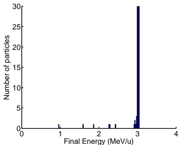
Figure 4: Histogram of output energy of the *FETS* 4-rod RFQ field simulation.
