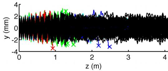
Figure 5: The trajectories of the model particles through the *FETS* 4-rod RFQ field simulation.
