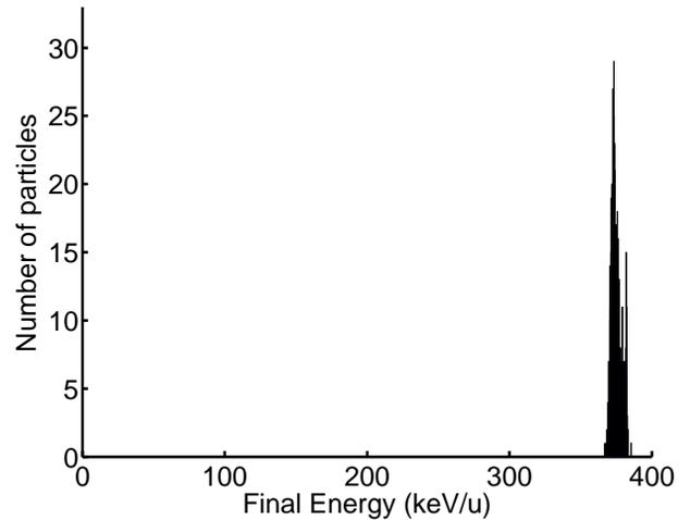
Figure 6: Histogram of output energy of carbon  $4^+$  ions in RFQ simulation set at 200 MHz and 2.4 m length with an input energy of 8 keV/u.
