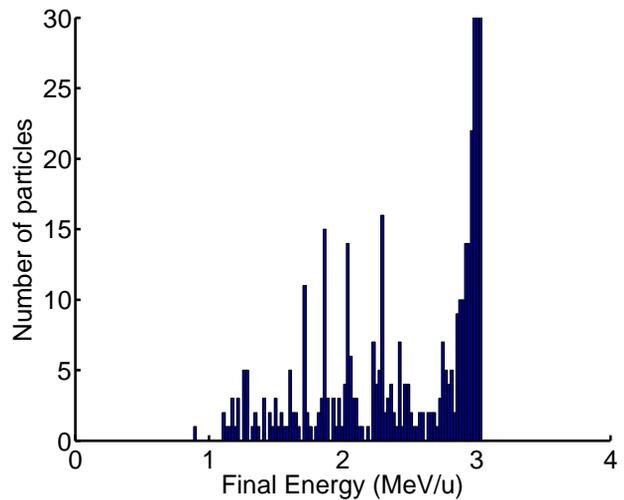
Figure 2: Histogram of output energy of the *FETS* 4-vane RFQ field simulation.
