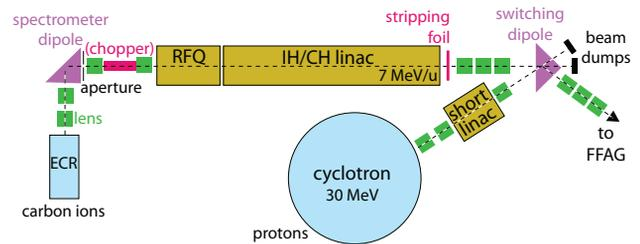
Figure 1: Schematic of proposed injector assembly, including ion sources, LEBT, pre-accelerators and MEBT. The proton source is contained within the cyclotron.
