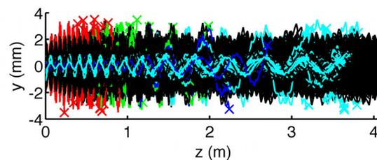
Figure 3: The trajectories of the model particles through the *FETS* 4-vane RFQ field simulation with particle tracks tagged by colour according to the end of the particle track.
