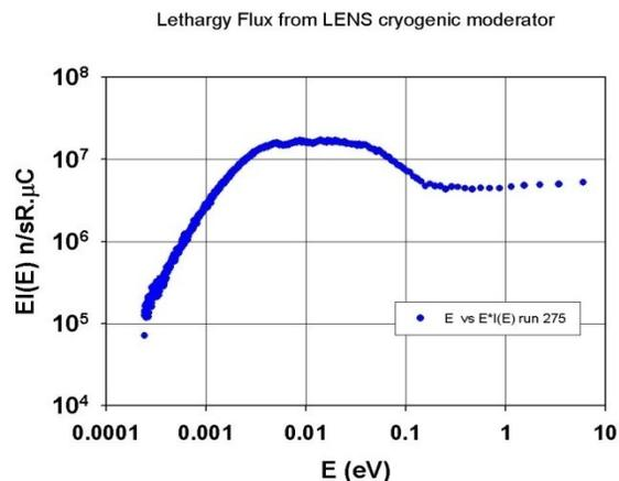
Figure 7: EMS measured neutron flux from the cryogenic methane moderator.
