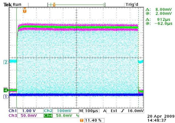
Figure 3: The 13 MeV Proton Beam Pulse as detected by 2 current transformers shown in red and green and an RF pickup shown in light blue.
