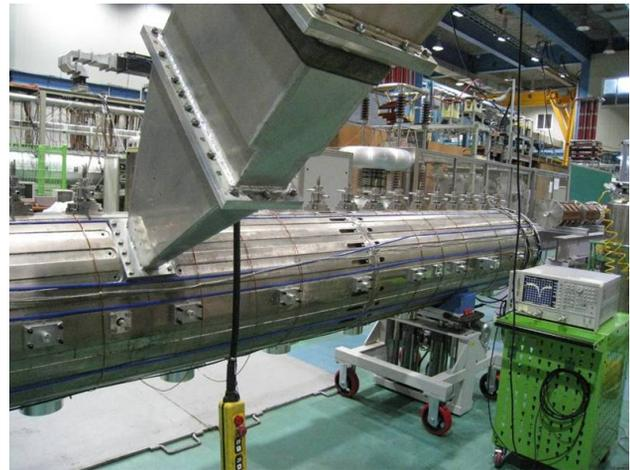
Figure 6: RF coupler cold model mounted on DTL.
