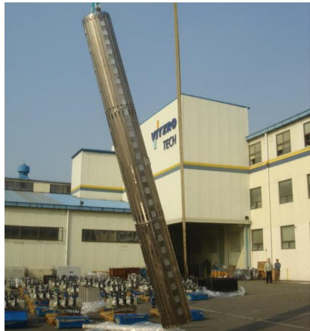
Figure 1: Three-section combined into one tank assembly.
