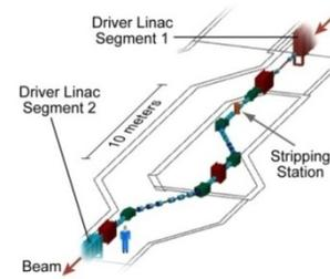
Figure 4: Layout of the Charge-Stripping Section.
