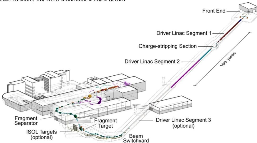
Figure 1: Layout of the FRIB Driver linac.
