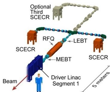
Figure 2: Layout of the FRIB driver linac front end.
