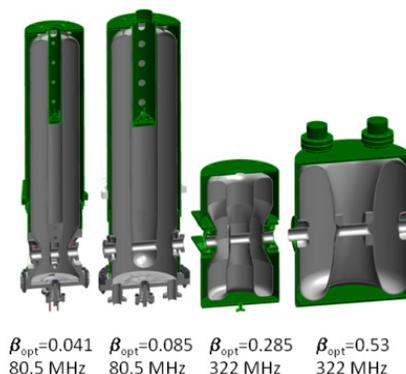
Figure 3: SC Quarter-Wave Resonators and Half-Wave Resonators used in FRIB SC linac Segments 1 and 2.
