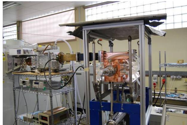
Figure 3: The ACLIP module high power RF test set.
