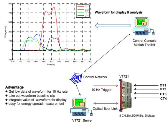
Figure 10: The block diagram of the CAEN V1721 digitizer for CT1, CT2, CT3 and CT4 waveform capture.
