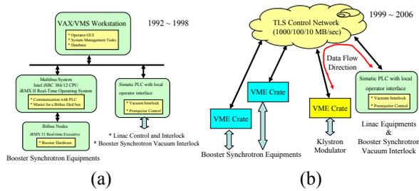
Figure 2: (a) Functional block diagram of the original turnkey control system. (b) System block diagram of renewed control system in 1998. The signal flow between PLC and VME crate is highlighted.
