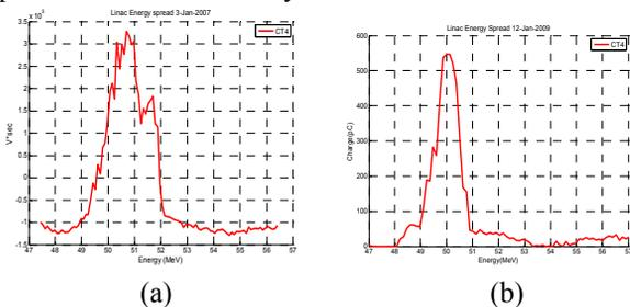
Figure 9: (a) The energy spread measurement in January 2007. (b) The energy spread reduces to less than 1 MeV (FWHM) in January 2009.
