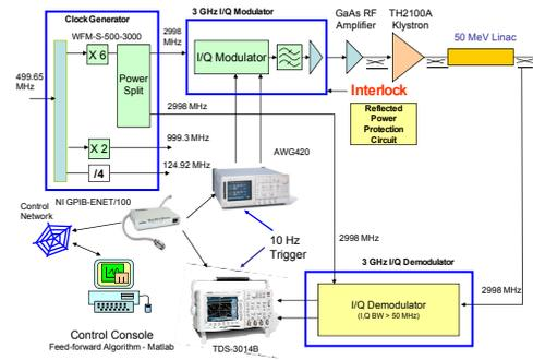
Figure 5: The block diagram of the low level RF system for the 50 MeV linear accelerator.
