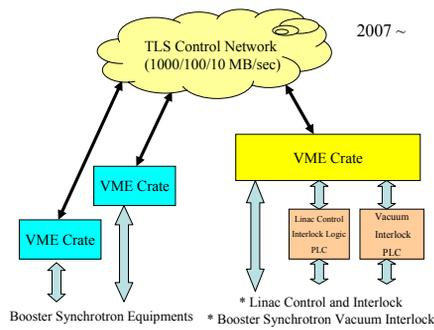
Figure 3: New control environment for linac system.
