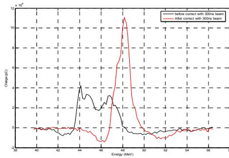
Figure 7: The RF amplitude and phase waveform before and after correction with bunch train length 300 nsec beam, energy spread is reduced simultaneously.
