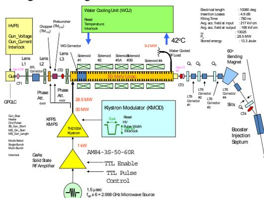
Figure 1: Synoptic of the 50 MeV linear accelerator system components of the TLS.
