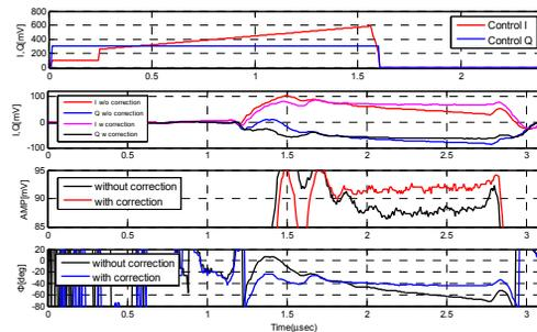
Figure 6: RF amplitude and phase waveform before and after correction with bunch train 600 nsec beam, both amplitude and phase are corrected simultaneously.
