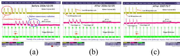
Figure 4: (a) Old control system with 0.3 ~0.4 second transmitting delay before December 2006. (b) The delay is reduced to less than 0.1 second after December 2006. (c) The new control system with modified timing control circuitry has not produced extra trigger pulse after May 2007.
