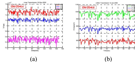
Figure 8: (a) The transmission of pre-injector in December 2006. (b) The transmission of pre-injector after updated of low level RF system in 2009.
