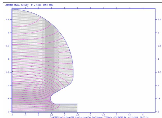
Figure 2: SuperFish plot of a single cell.
