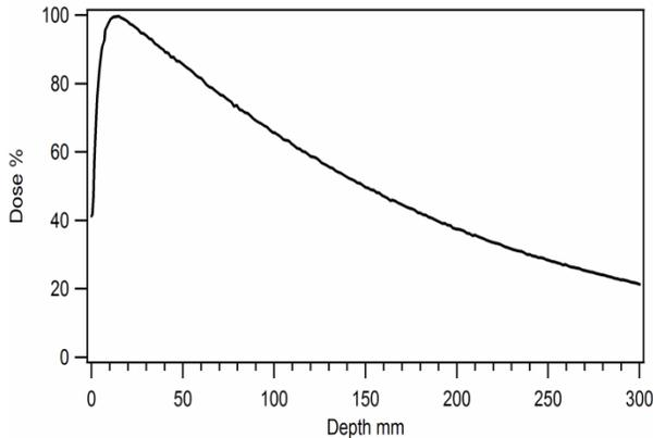
Figure 5: Measured depth dose curve in water.
