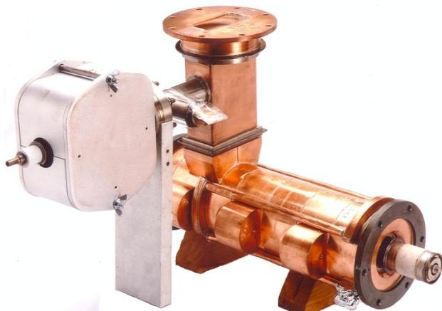
Figure 3: SAMEER made side coupled linac tube.
