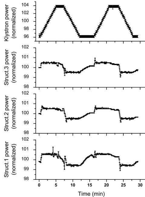
Figure 4: RF power at the structures as a function of time, while the klystron power (top plot) is changed.
