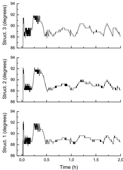
Figure 3: Phase difference in the first three accelerating structures, indicating the resonance condition.
