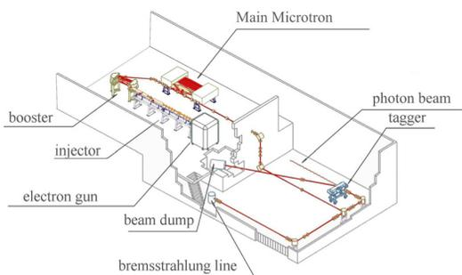
Figure 1: View of the IFUSP microtron.
