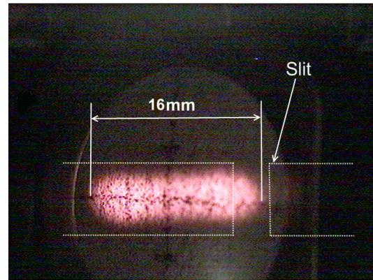
Figure 7: Beam deflected horizontally after the first chopper cavity. The dotted points indicate the slit behind this view-screen.
