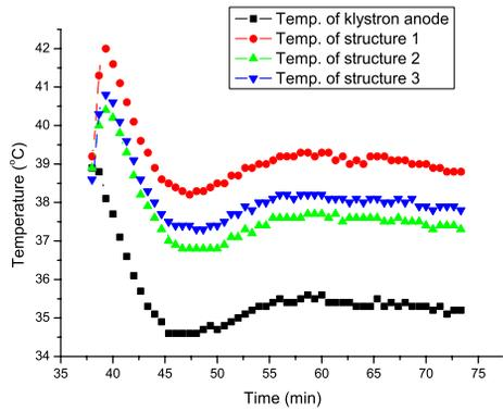
Figure 2: Temperature behavior as a function of time. The plot begins when the RF is applied to the first three accelerating structures.
