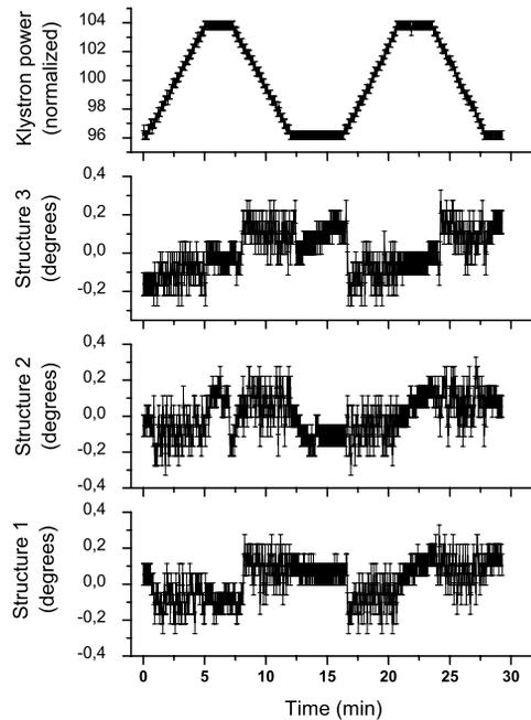
Figure 5: RF phase at the structures as a function of time, while the klystron power (top plot) is changed.
