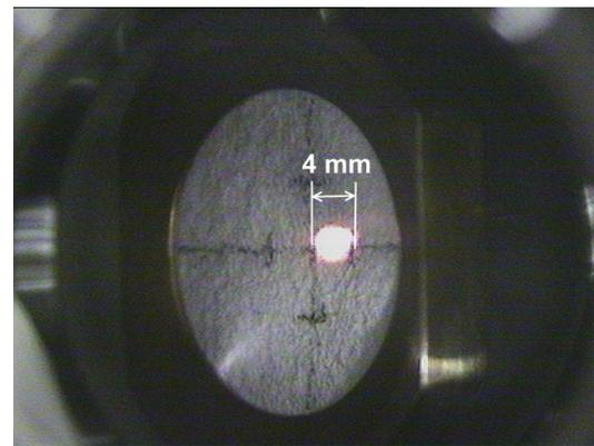
Figure 8: Beam after the chopper and buncher cavities.
