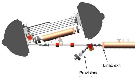
Figure 6: Provisional beam line to allow energy measurements.
